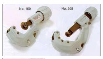
Features an enclosed feed screw to eliminate clogging and jamming, groved rolls for close-to-flare cuts, and a fold-away reamer. Made from high-strength aluminum alloy with a spare cutter in the handle. Cuts copper, brass, and aluminum tubing, and thin-wall conduit. Model 205 has all the features of the No. 150, plus a quick-acting mechanism.
