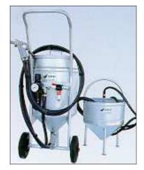
Thanks to its easiness of handling and using, the Abro-Jet blast machine is adapted to the cleaning of any type of materials (iron, aluminium, glass, wood, stone...).
