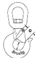
Swivel hook dimensions with PL latch assembled
